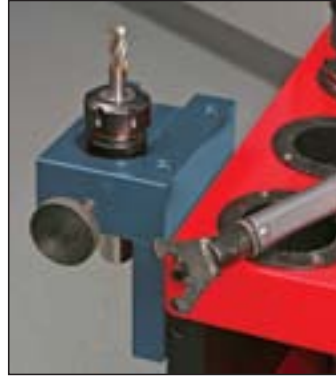
A large set-screw engages the drive slot in BT and CAT holders.
