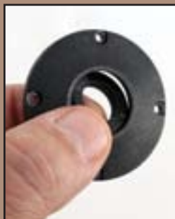
Insert Black Gold coolant ring into cap
