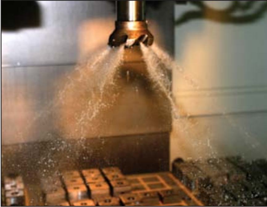
CoolBLAST arbor screw provides coolant path.
