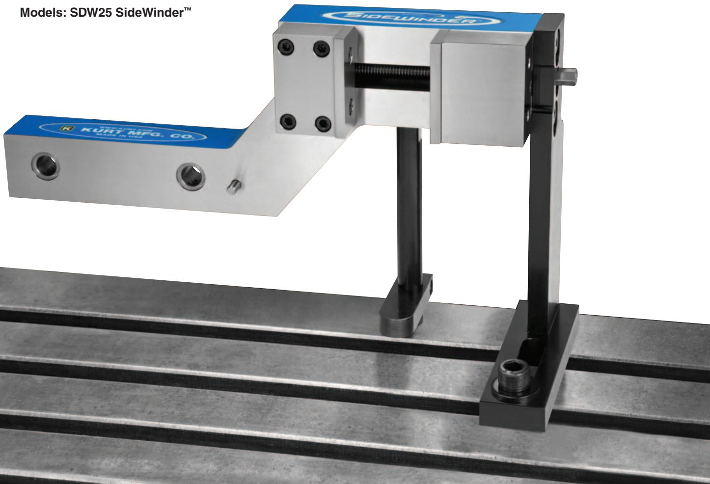
The Kurt SideWinder is a vise that mounts vertically to the back of any Kurt 6" vise with an integral bracket. The bracket will include a stabilization leg that will mount to the table on the movable end of the vise and a workstop to position the height of the part.
